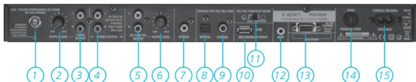
1. **Antenna connector:** connect the antenna supplied here. Do not connect this to a cable distribution network, unless you use an isolation transformer. Connecting the unit to a cable network may cause interference to the DAB reception. This depends on the signal present on the cable network. Check availability of DAB signals with the cable network supplier first!
